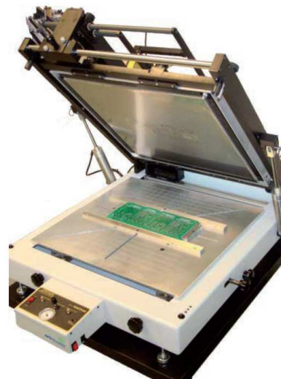
Dual cameras provide axial vision alignment of the PCB board to the stencil for precise delivery of solder paste.
