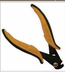
A manual depaneling tool to separate larger sheets of multiple PCB panels in a quick, economic and safe way, leaving well finished cut surfaces; maximum length of the isthmus (tab) must not exceed 2.5 mm.
