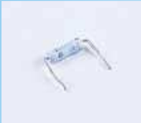
48.0L01 CUT BEND AND FLATTEN LEADS
