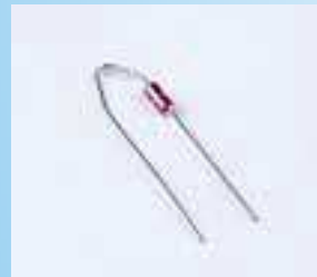
SP22.21 CUT AND BEND FOR VERTICAL MOUNT
